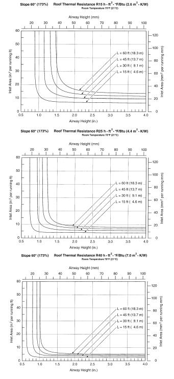
Figure 10 Airway heights and inlet areas for cathedral ceilings with a slope of 60°.
