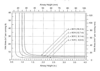
Figure 9 Airway heights and inlet areas for cathedral ceilings with a slope of 45°.
