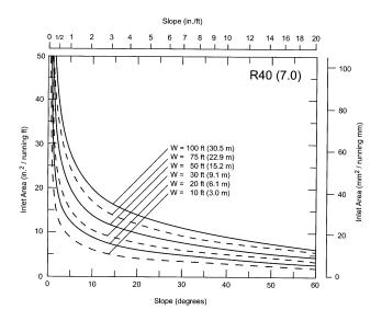
*Figure 5* Net free open area of inlets for attics with R40 (in SI units, R7.0) insulation.
