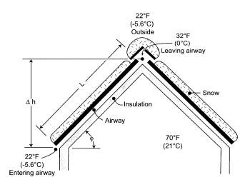
Figure 6 A typical ventilated cathedral ceiling.
