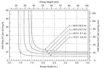
Slope 30° (58%) Roof Thermal Resistance R40 h • ft<sup>2</sup> • °F/Btu (7.0 m<sup>2</sup> • K/W) Boom Temperature 70°F (21°C
