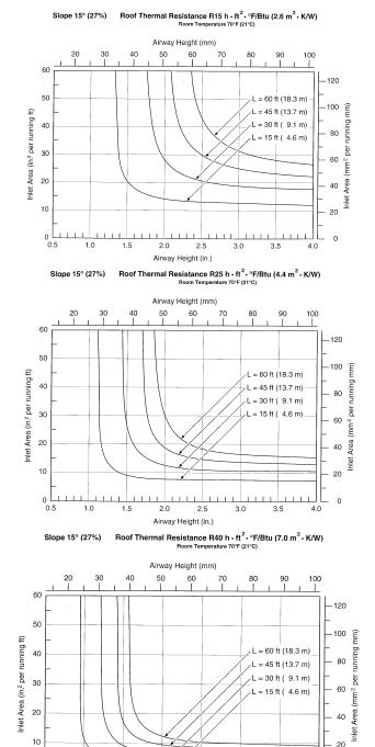
Figure 7 Airway heights and inlet areas for cathedral ceilings with a slope of 15°.
