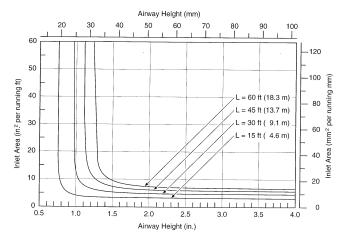
Figure 8 Airway heights and inlet areas for cathedral ceilings with a slope of 30°.
