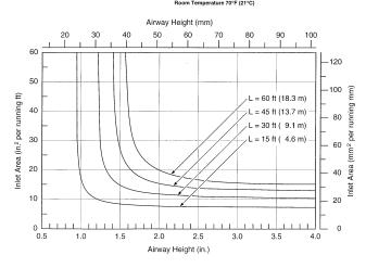
Slope 45° (100%) Roof Thermal Resistance R25 h • ft<sup>2</sup> • °F/Btu (4.4 m<sup>2</sup> • K/W) Room Temperature 70°F (21°C)
